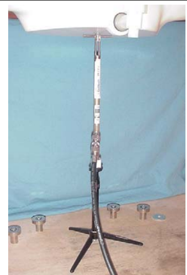
1900 MHz Validation Dipole Setup
