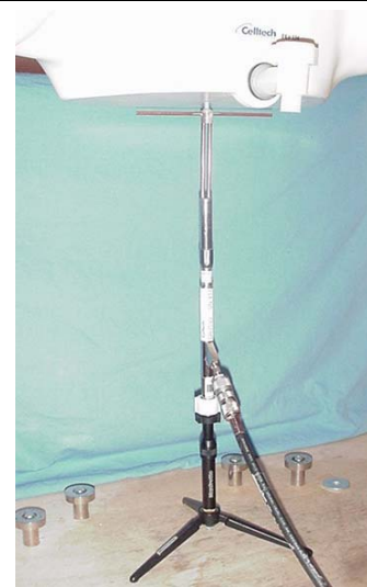
835 MHz Validation Dipole Setup
