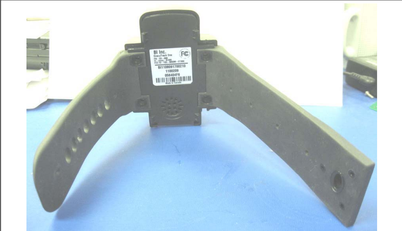
DUT with Back Plate Removed showing Metal Mounting Screws for Ankle Strap Attachment
