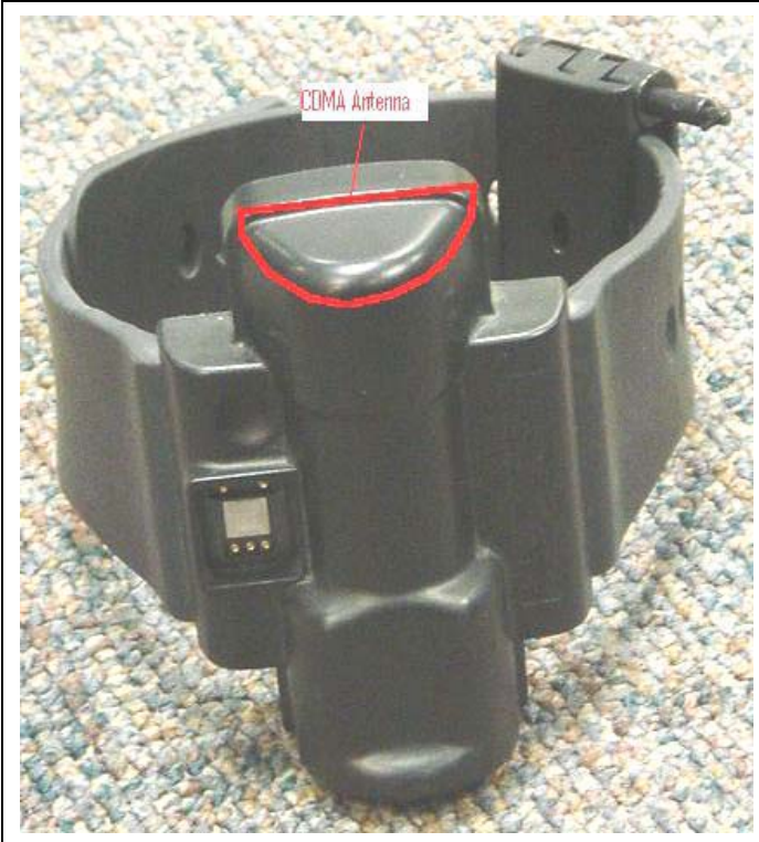
Outer Facing Surface of DUT and Antenna Location
