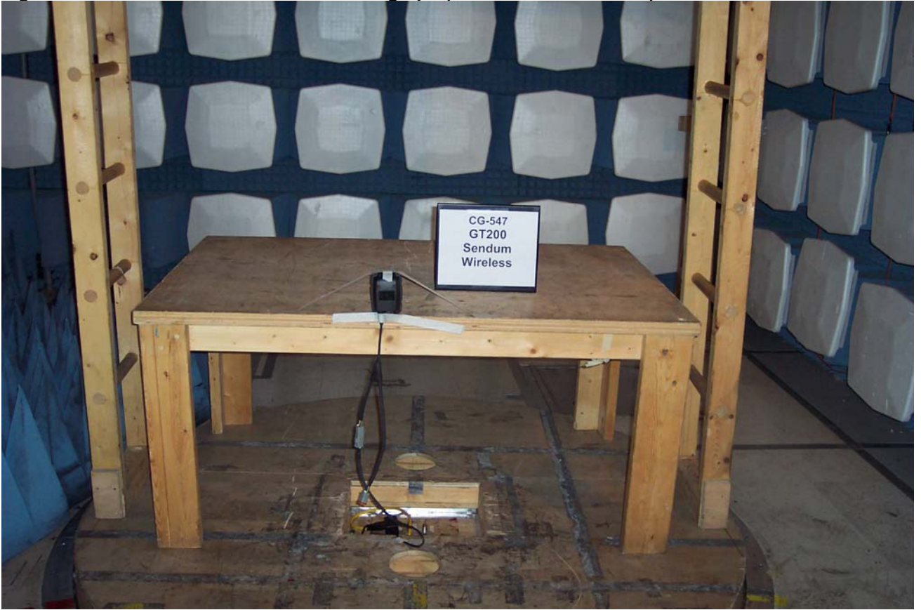
Figure 1 Radiated Emissions Test Photograph (worst case orientation)
