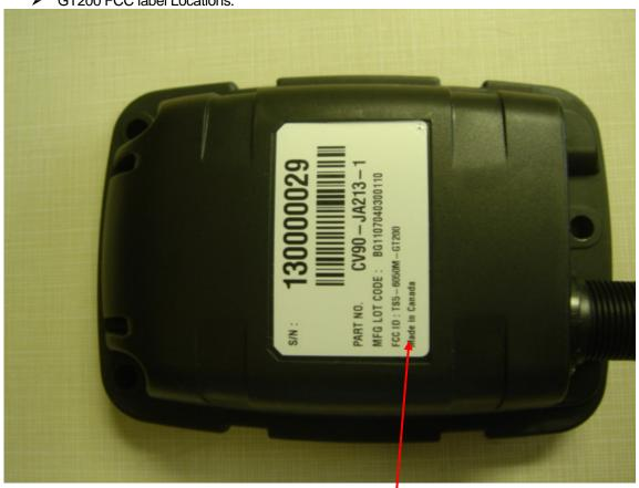
The IC number will be placed on the label underneath the FCC ID number. The model number: GT200 will be placed underneath the Part Number
