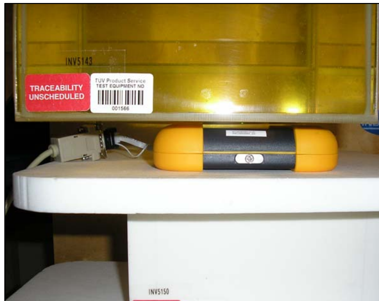
Figure 17: Positional Photograph of the Arcom Cyber Tracker Device in Rear Facing Phantom Position (Side View)
