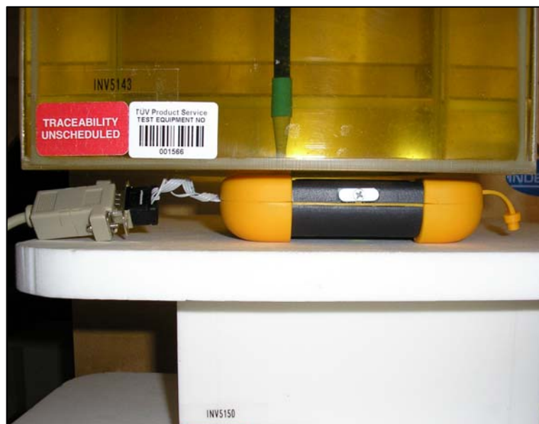
Figure 15: Positional Photograph of the Arcom Cyber Tracker Device in Front Facing Phantom Position (Side View)
