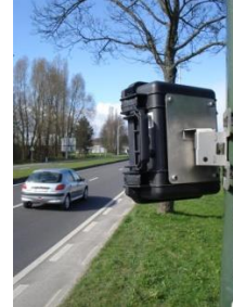
Figure 5: radar installed on the pole bracket
