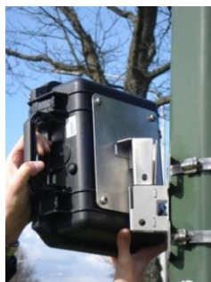
Figure 6: place the radar on its bracket
