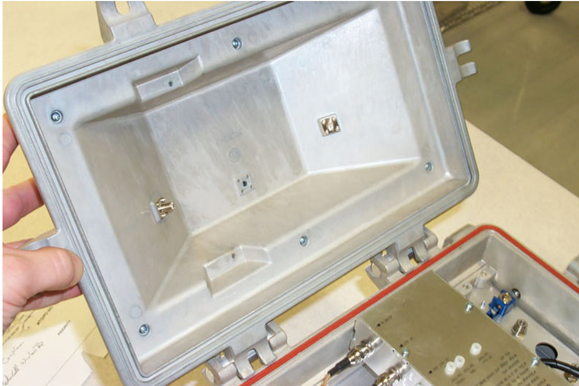
Figure 23 Antenna inside cover of EUT
