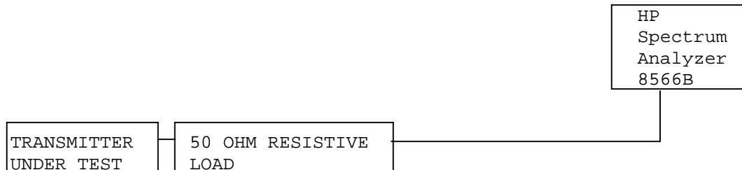
**METHOD OF MEASUREMENT:** The procedure used was TIA/EIA-603 STANDARD without any exceptions. The measurements were made at TIMCO ENGINEERING INC. 849 N.W. State Road 45, Newberry, Florida 32669.
