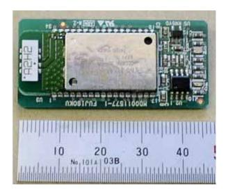
(5) Removed shield Case of the RF (Bluetooth) Module
