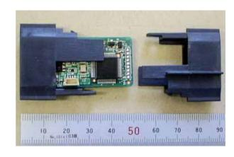
(3) Removed both of Outer Cover (Bottom View)
