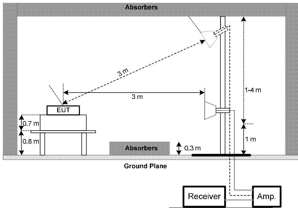
(C) For radiated emissions below 30MHz
