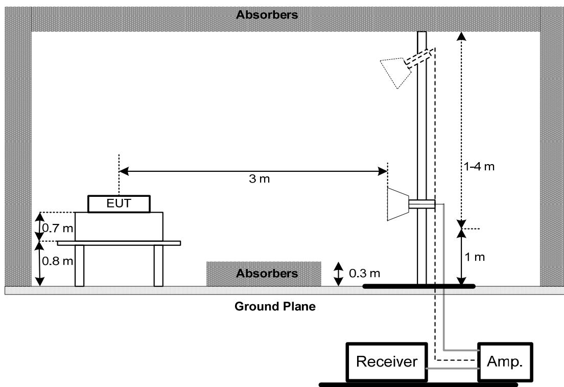
(C) For radiated emissions below 30MHz
