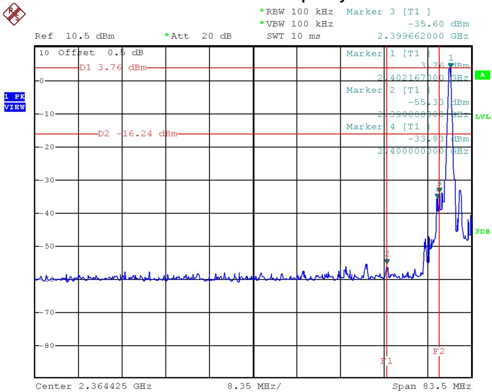
**Bluetooth / 1 Mbps / CH78-The max. radio frequency power in any 100 kHz bandwidth within the frequency band**
