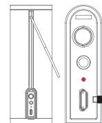
To Charge X6, connect X6 with computer through a Micro USB cable. The Power LED will flash red light when charging and turn solid light after full charging.
