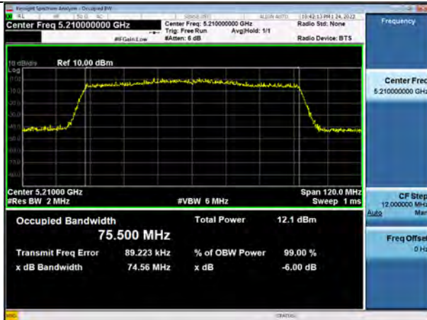
802.11ac_VHT80 UNII 2C BAND 99 % Bandwidth(CH 106)
