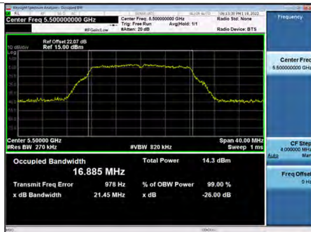
802.11a UNII 2C BAND 26 dB Bandwidth (CH100)
