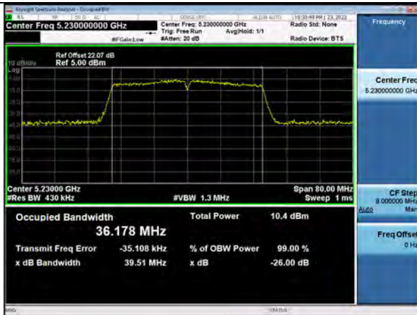
802.11n_HT40 UNII 1 BAND 26 dB Bandwidth(CH 46)
