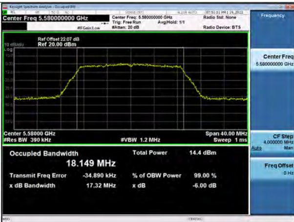
802.11ac_VHT20 UNII 2C BAND 99 % Bandwidth(CH 116)
