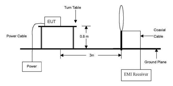
The diagram below shows the test setup that is utilized to make the measurements for emission from 30 Mb to 1 Gb Emissions.
