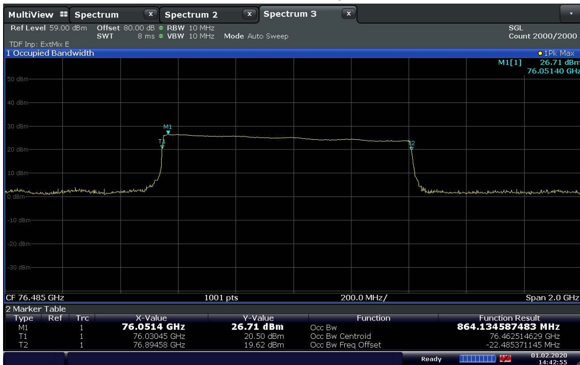
Occupied Bandwidth plot (High Resolution)
