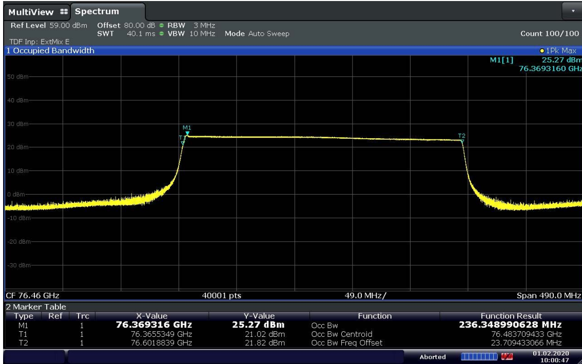
Occupied Bandwidth plot (High Resolution)
