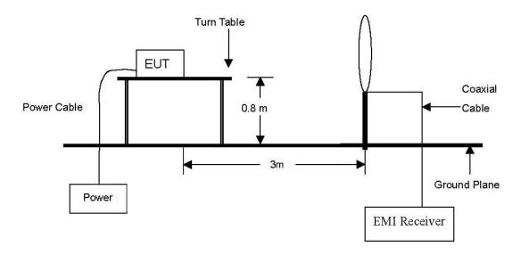
The diagram below shows the test setup that is utilized to make the measurements for emission from 30  $\,\rm Me$  to 1  $\,\rm Gh$ .
