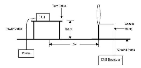
The diagram below shows the test setup that is utilized to make the measurements for emission from 30 Mz to 1  $\mathbb{G}_2$  Emissions.
