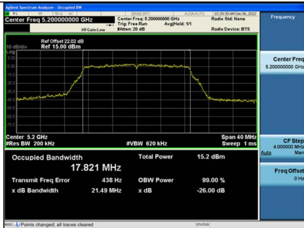
802.11ac_VHT20 UNII 2C BAND 26 dB Bandwidth(CH 144)
