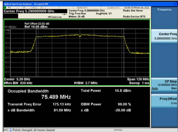
802.11ac_VHT80 UNII 3 BAND 26 dB Bandwidth (CH 155)
