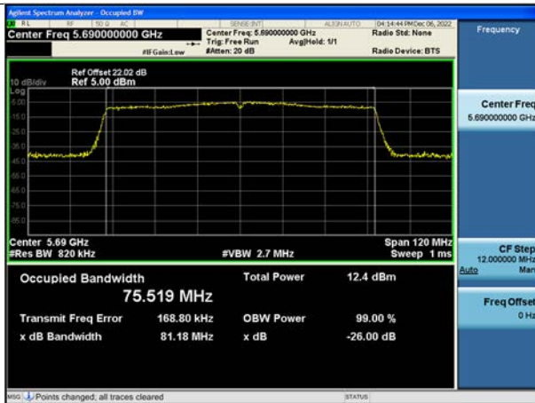
802.11ac_VHT80 UNII 2C BAND 26 dB Bandwidth(CH 138)
