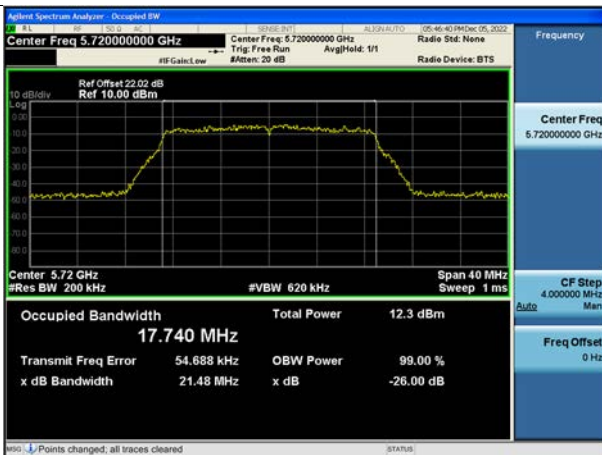
802.11n_HT20 UNII 2C BAND 26 dB Bandwidth(CH 144)
