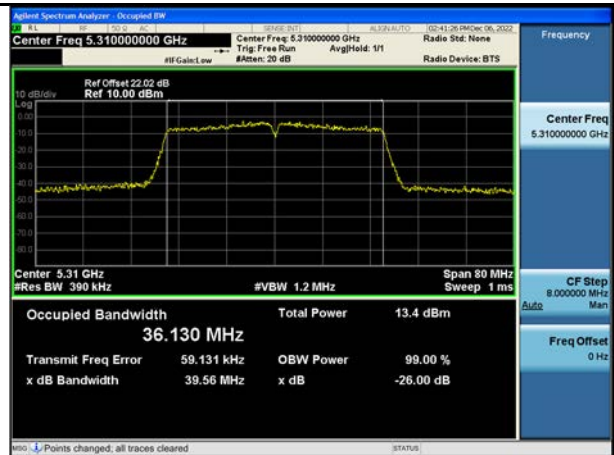
802.11n_HT40 UNII 3 BAND 26 dB Bandwidth (CH 151)
