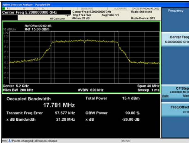
802.11n_HT20 UNII 2C BAND 26 dB Bandwidth(CH 144)
