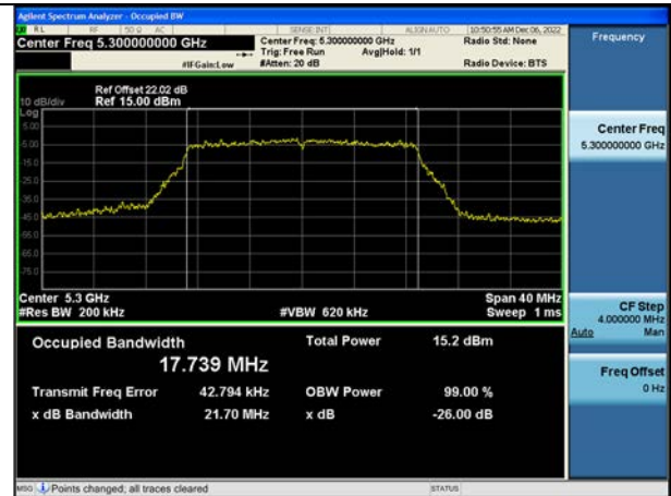
802.11ac_VHT20 UNII 3 BAND 26 dB Bandwidth(CH 165)
