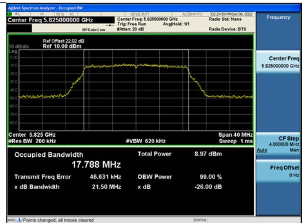
802.11ac_VHT20 UNII 3 BAND 26 dB Bandwidth(CH 165)
