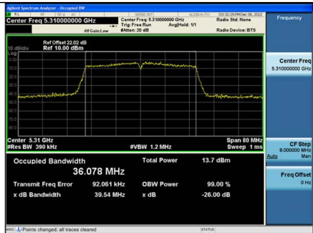
802.11ac_VHT40 UNII 3 BAND 26 dB Bandwidth (CH 151)
