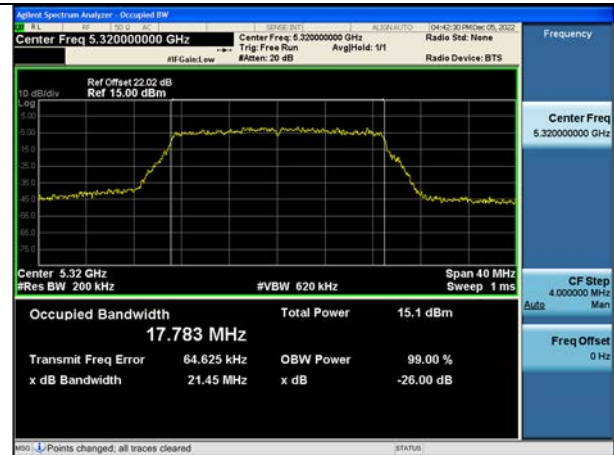
802.11n_HT20 UNII 3 BAND 26 dB Bandwidth(CH 165)
