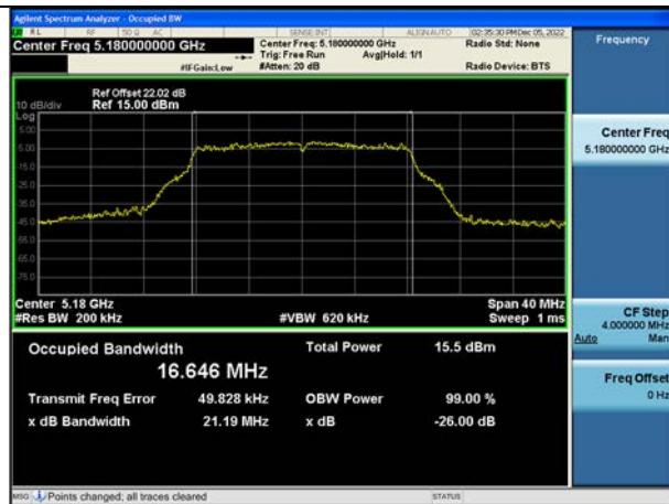
802.11a UNII 2C BAND 26 dB Bandwidth (CH 100)
