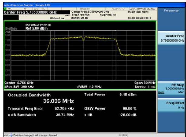
802.11n_HT40 UNII 3 BAND 26 dB Bandwidth (CH 151)
