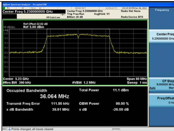
802.11ac_VHT40 UNII 2C BAND 26 dB Bandwidth(CH 102)
