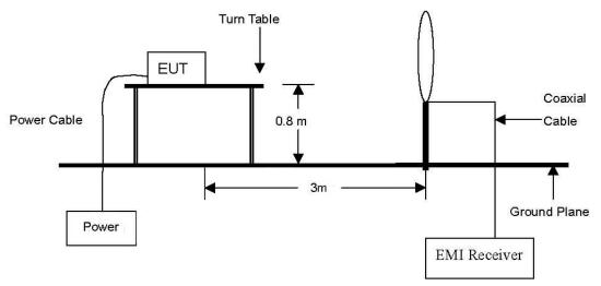
The diagram below shows the test setup that is utilized to make the measurements for emission from 30 ML to 1 GHz emissions.
