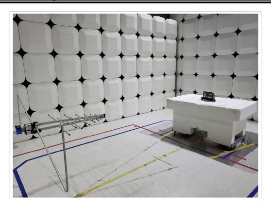
Test Setup Photo of Radiated Measurement (Below 1GHz)
