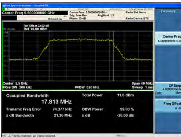
802.11ac_VHT20 UNII 2C BAND 99 % Bandwidth(CH 100)
