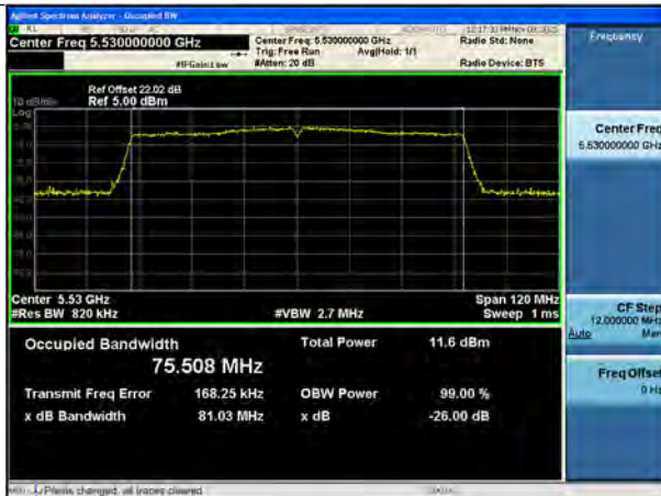
802.11ac_VHT80 UNII 2C BAND 26 dB Bandwidth(CH 106)
