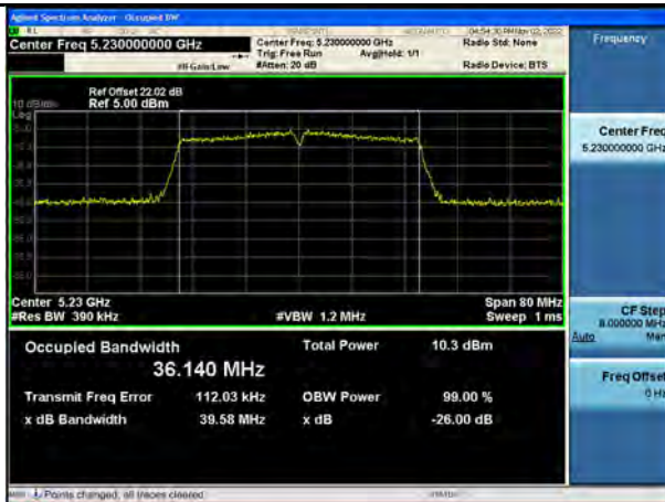
802.11n_HT40 UNII 2C BAND 99 % Bandwidth(CH 102)
