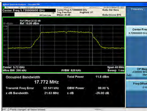
802.11ac_VHT20 UNII 2C BAND 26 dB Bandwidth(CH 144)
