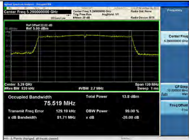
802.11ac_VHT80 UNII 3 BAND 26 dB Bandwidth (CH 155)
