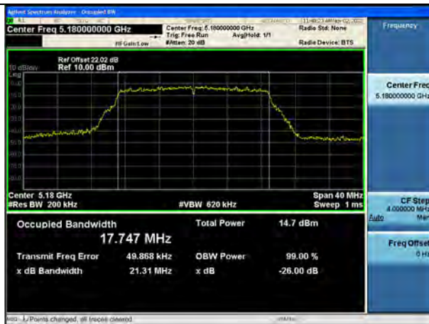
802.11ac_VHT20 UNII 2C BAND 26 dB Bandwidth(CH 144)
