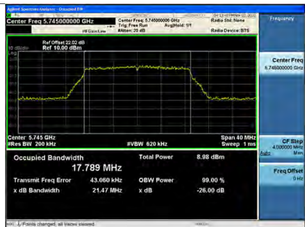
802.11ac_VHT20 UNII 3 BAND 26 dB Bandwidth(CH 149)
