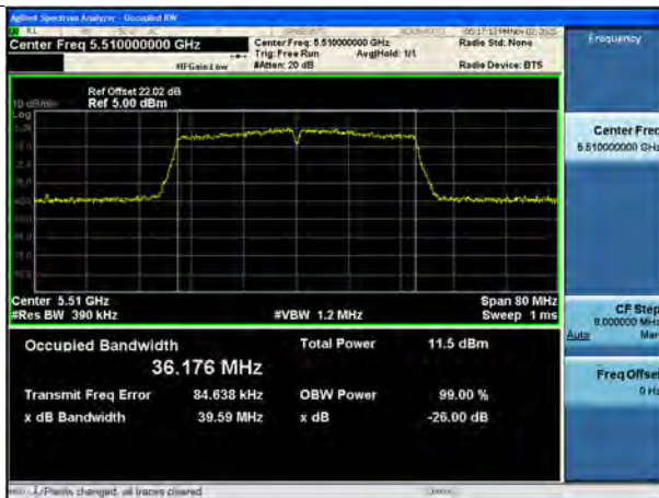
802.11n_HT40 UNII 2C BAND 99 % Bandwidth(CH 102)
