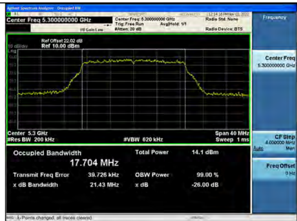
802.11ac_VHT20 UNII 3 BAND 26 dB Bandwidth(CH 149)
