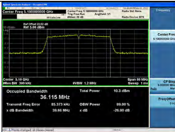
802.11n_HT40 UNII 2C BAND 26 dB Bandwidth(CH 102)
