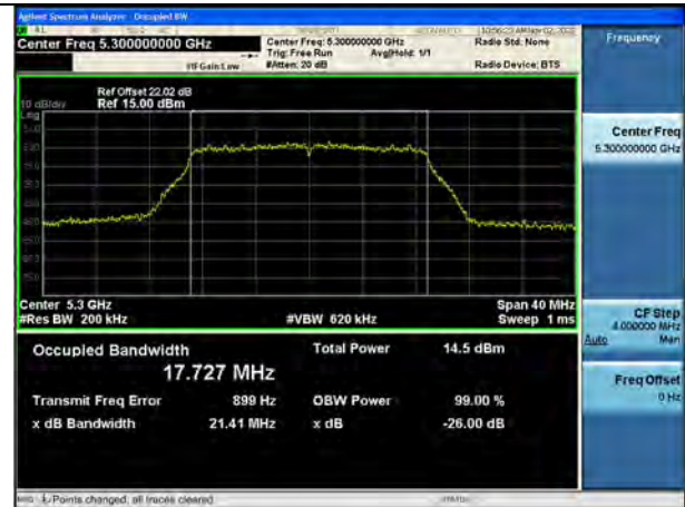
802.11n_HT20 UNII 3 BAND 26 dB Bandwidth(CH 149)
