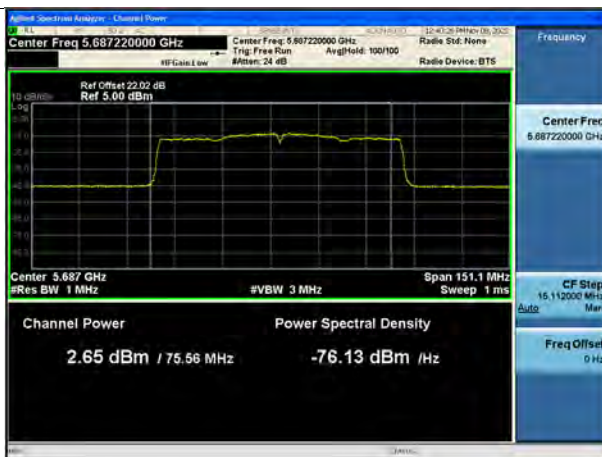
802.11ac(VHT80) UNII 2C Band
