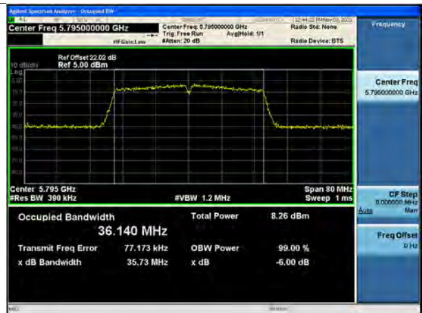
802.11n_HT40 UNII 3 BAND 99 % Bandwidth (CH 159)
