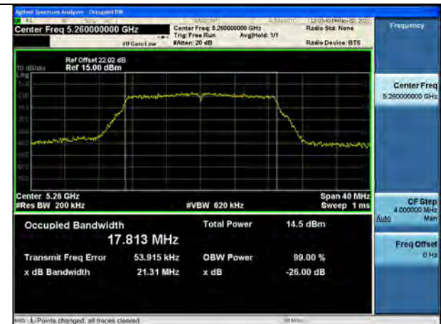
802.11ac_VHT20 UNII 3 BAND 99 % Bandwidth(CH 157)
