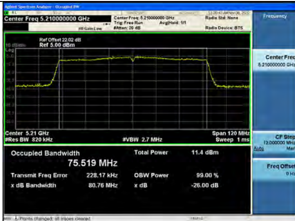
802.11ac_VHT80 UNII 2C BAND 26 dB Bandwidth(CH 106)
