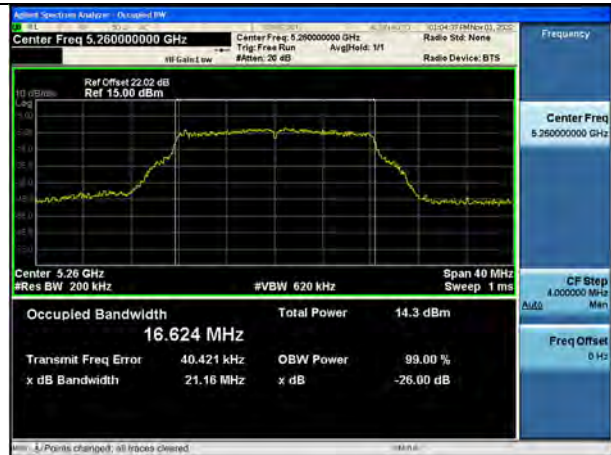
802.11a UNII 3 BAND 26 dB Bandwidth (CH 165)
