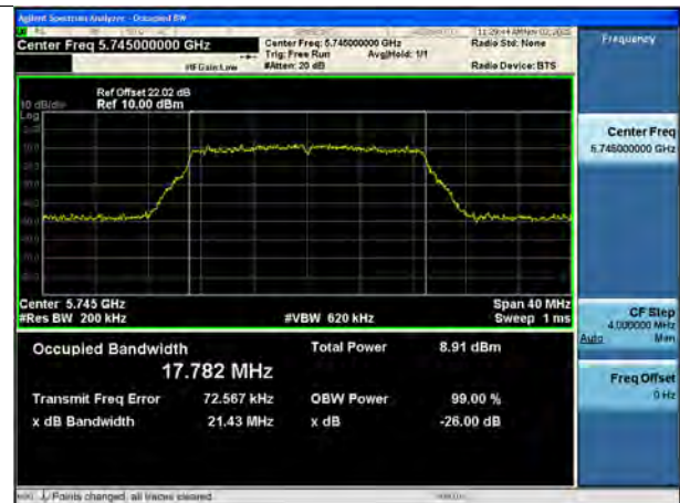
802.11n_HT20 UNII 3 BAND 26 dB Bandwidth(CH 149)
