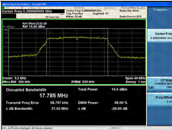
802.11n_HT20 UNII 2C BAND 26 dB Bandwidth(CH 100)
