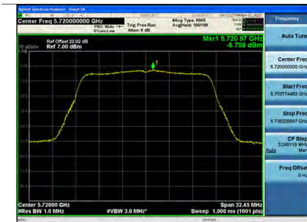
802.11ac(VHT20) UNII 2C Band
