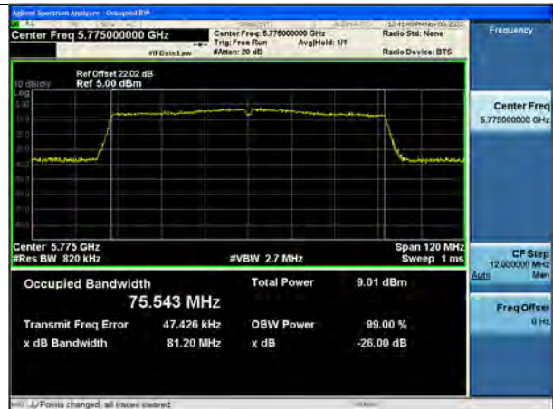
802.11ac_VHT80 UNII 3 BAND 26 dB Bandwidth (CH 155)
