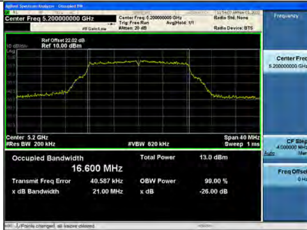
802.11a UNII 2C BAND 99 % Bandwidth (CH 144)
