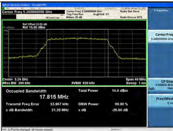
802.11ac_VHT20 UNII 2C BAND 99 % Bandwidth(CH 100)
