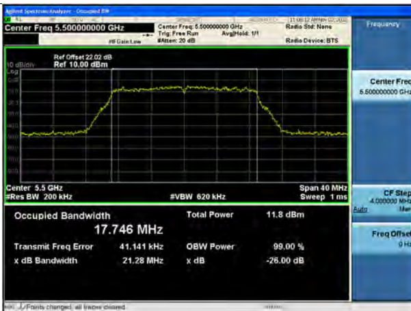
802.11n_HT20 UNII 2C BAND 26 dB Bandwidth(CH 100)
