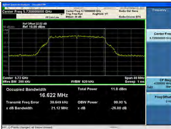
802.11a UNII 2C BAND 26 dB Bandwidth (CH 144)
