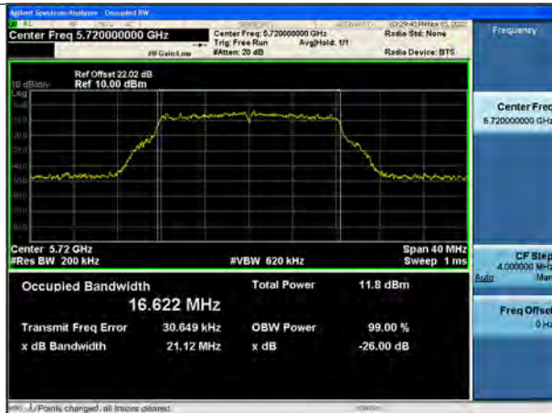
802.11a UNII 2C BAND 99 % Bandwidth (CH 144)
