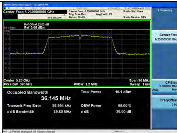
802.11ac_VHT40 UNII 2C BAND 26 dB Bandwidth(CH 102)
