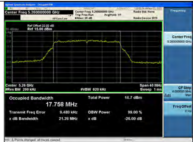
802.11n_HT20 UNII 3 BAND 99 % Bandwidth(CH 149)
