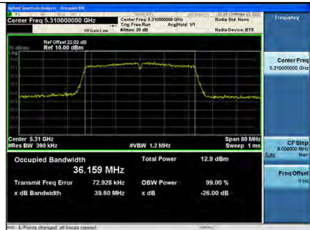
802.11ac_VHT40 UNII 3 BAND 26 dB Bandwidth (CH 151)
