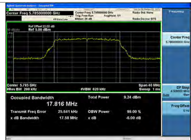
802.11ac_VHT20 UNII 3 BAND 99 % Bandwidth(CH 157)
