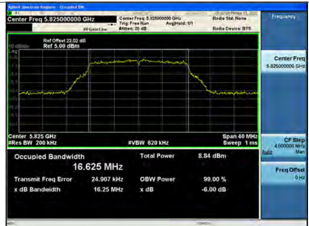
802.11a UNII 3 BAND 99 % Bandwidth (CH 165)
