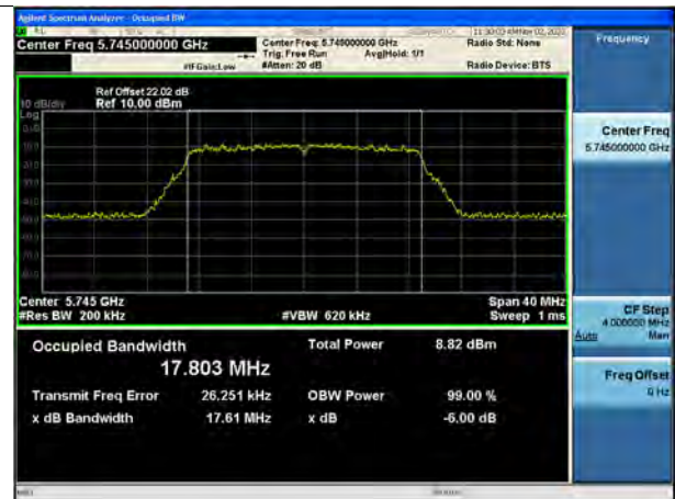
802.11n_HT20 UNII 3 BAND 99 % Bandwidth(CH 149)
