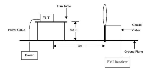
The diagram below shows the test setup that is utilized to make the measurements for emission from 30 Mz to 1  $\mathbb{G}_{\mathbb{Z}}$ .
