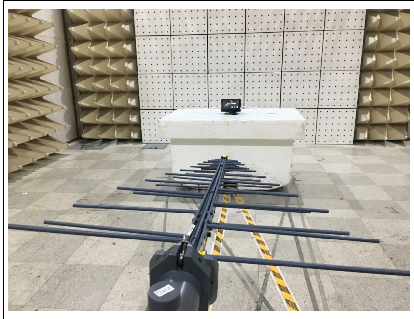
3. Photo of Radiated Spurious Emission Test (Above 1 GHz)
