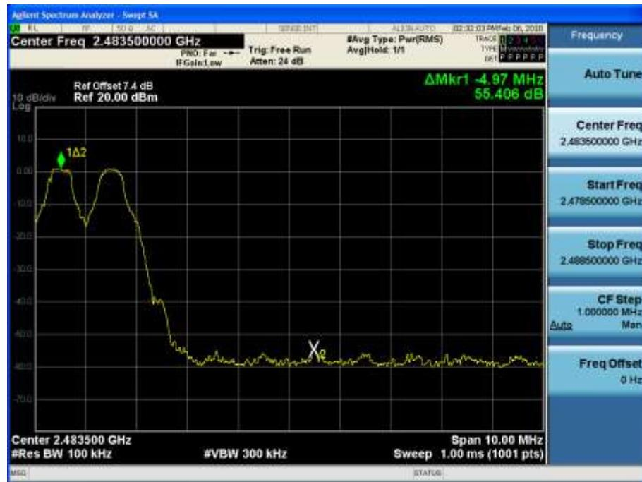
Test Plots with hopping (8DPSK)
