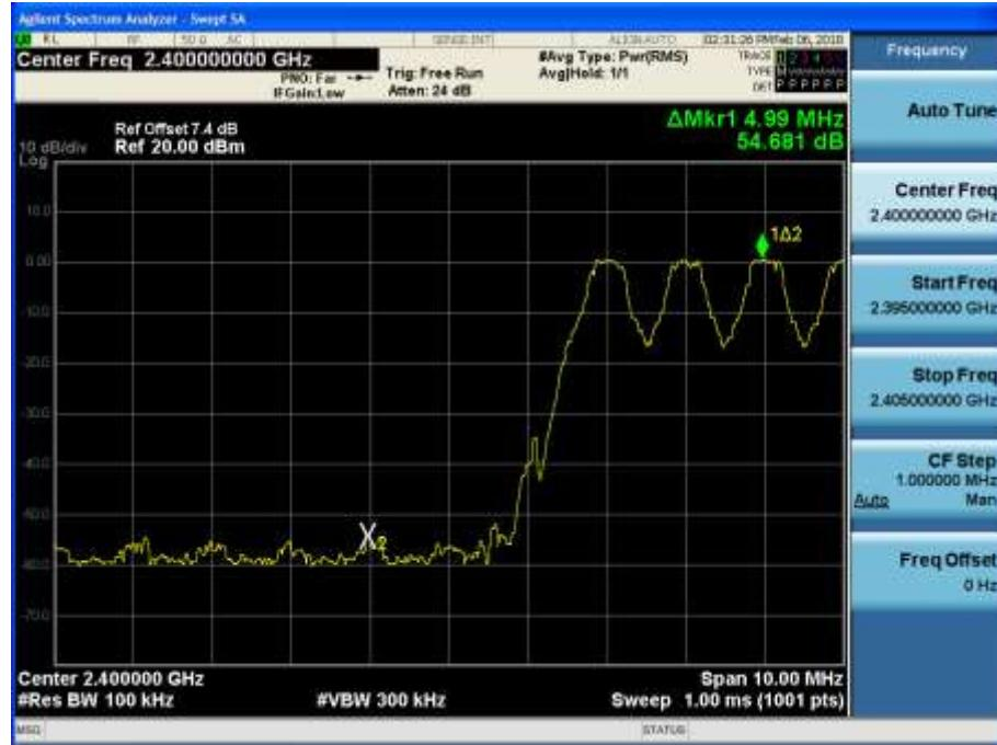
Test Plots with hopping (GFSK)
