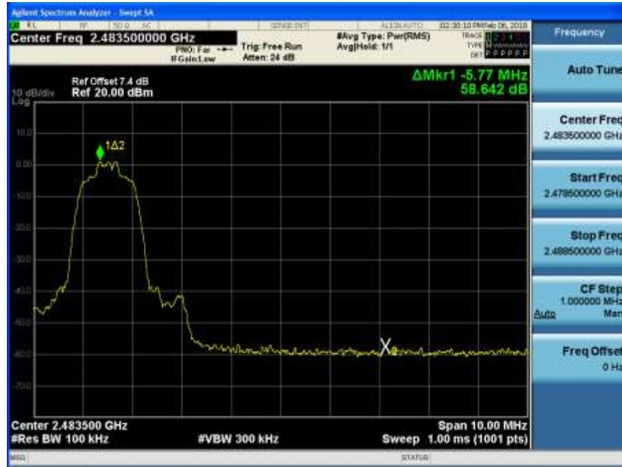
Test Plots with hopping (GFSK)
