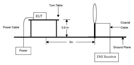
The diagram below shows the test setup that is utilized to make the measurements for emission from 30  $\,{\rm Mz}$  to 1  $\,{\rm Gz}$
