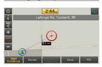
Touch the compass arrow icon to toggle between a map oriented to the North, oriented parallel to the vehicle's heading and 3D View.
