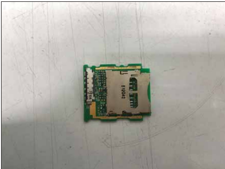
Bottom view of Sub PCB5
