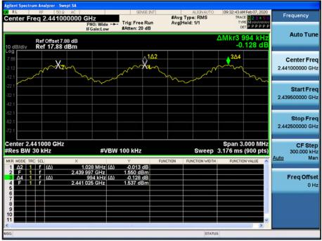
Test Plots (8DPSK) Channel Separation
