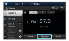
In the HD mode, HD Radio station buttons are displayed at the top of the radio screen. Touch a button to select one of the available HD Radio stations.
