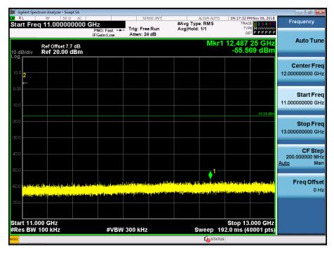
Test Plots (GFSK)- 13 GHz – 15 GHz Spurious Emission (CH.39)
