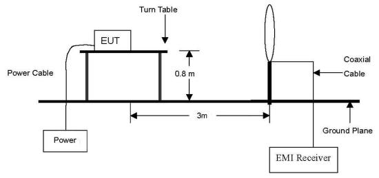
The diagram below shows the test setup that is utilized to make the measurements for emission from 30 Mz to 1  $\mathbb{G}_{\mathbb{Z}}$  emissions.
