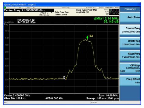
Test Plots without hopping (8DPSK) Band Edges (CH.78)
