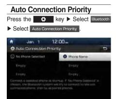
When the engine is running, the selected Bluetooth device is automatically connected. If you fail to connect the selected device, the previously-connected device is automatically connected, and if it also fails, then it tries to connect all paired devices sequentially.
