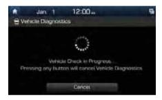
You can have your vehicle inspected only after stopping the vehicle because some control units can't be diagnosed while driving.
