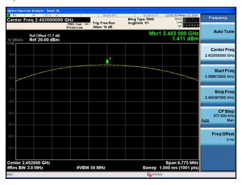
Test Plots (π/4DQPSK) Peak Power (CH.39)
