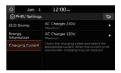
The Charging Current for AC Charger 240V mode and AC Charger 120V mode can be set.
