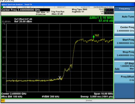
Test Plots with hopping (8DPSK)
