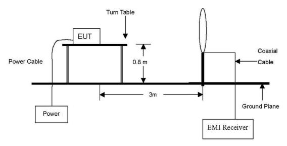
The diagram below shows the test setup that is utilized to make the measurements for emission from 30 Mz to 1  $\oplus$  emissions.
