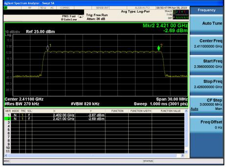
Number of Hopping Frequencies 1(AFH) <u>Hopping mode : Enable & 8DPSK</u>
