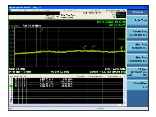
Conducted Spurious Emissions <u>Lowest Channel & Modulation : GFSK</u>
