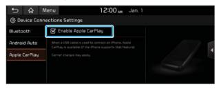
2 Connect an iPhone to the multimedia USB port on the vehicle by using the provided USB cable.
