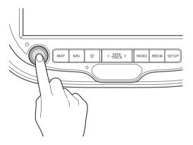
To shut down the system completely, park the vehicle in a safe place and stop the engine. The system automatically shuts down.
