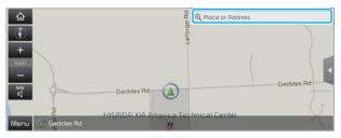
The **Place or Address** field appears only when the transmission shift lever is in the "P" (Park) position.
