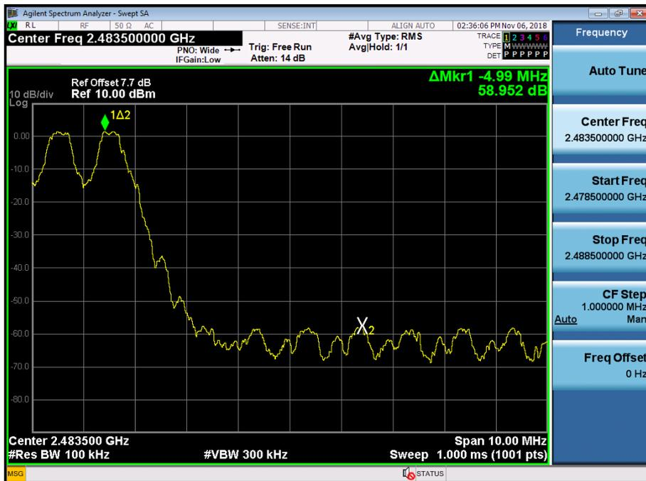
Test Plots with hopping (8DPSK)
