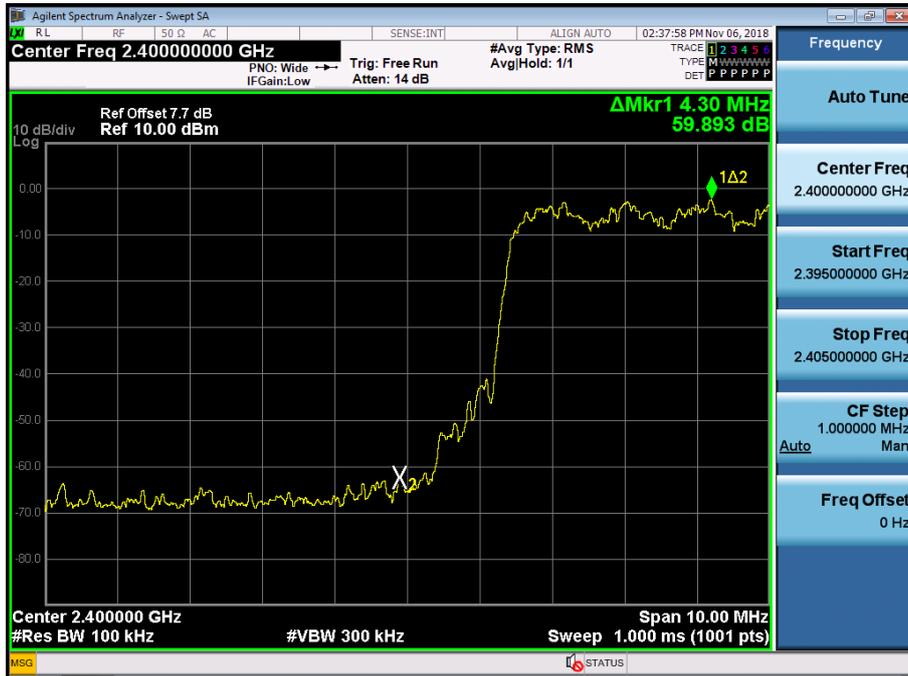
Test Plots with hopping (8DPSK)
