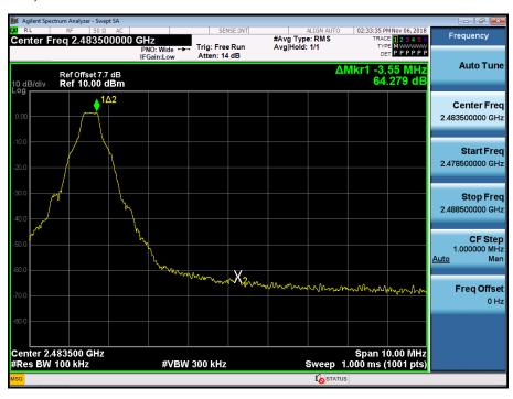
Test Plots without hopping (8DPSK) Band Edges (CH.0)
