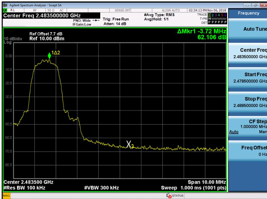
Test Plots with hopping (GFSK)
