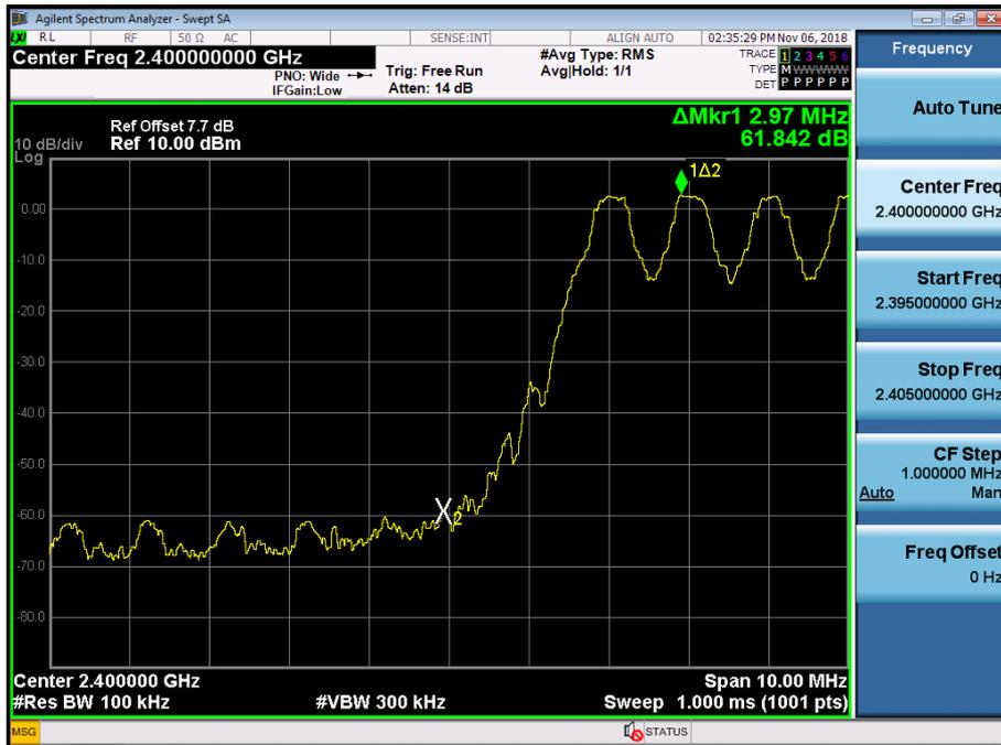
Test Plots with hopping (GFSK)
