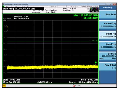
Test Plots (GFSK)- 13 GHz – 15 GHz Spurious Emission (CH.0)
