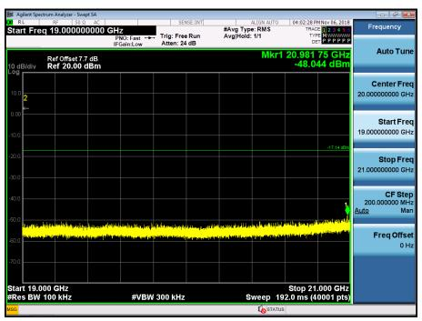
Test Plots (GFSK)- 21 GHz - 23 GHz Spurious Emission (CH.0)
