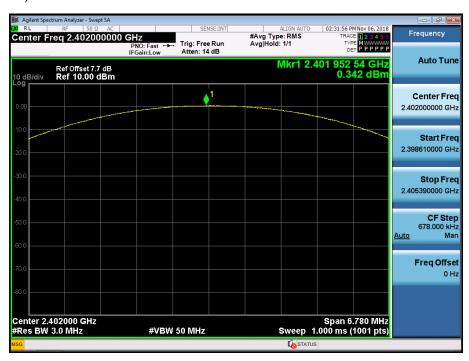
Test Plots (π/4DQPSK) Peak Power (CH.39)
