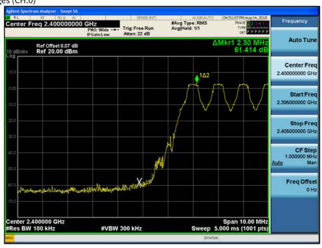
Test Plots with hopping (GFSK)
