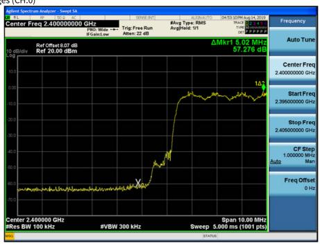
Test Plots with hopping ( $\pi/4DQPSK$ )
