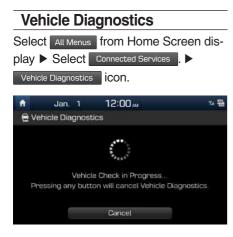
You can have your vehicle inspected only after stopping the vehicle because some control units can't be diagnosed while driving.
