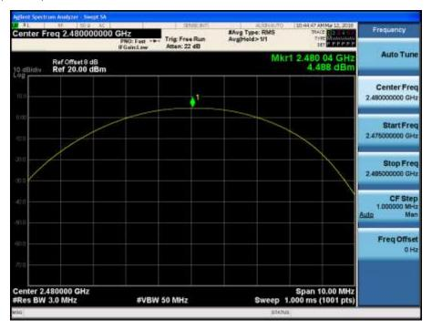
Test Plots (8DPSK) Peak Power (CH.0)
