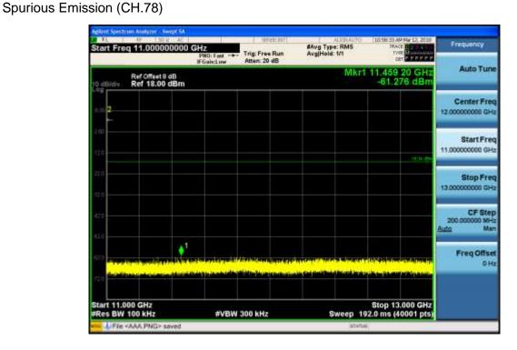
Test Plots (8DPSK)- 13 GHz – 15 GHz Spurious Emission (CH.78)
