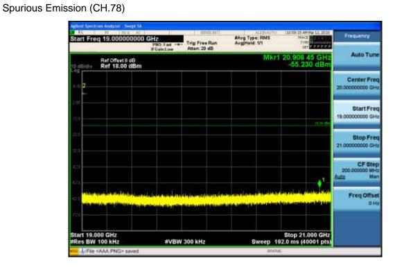
Test Plots (8DPSK)- 21 GHz - 23 GHz Spurious Emission (CH.78)
