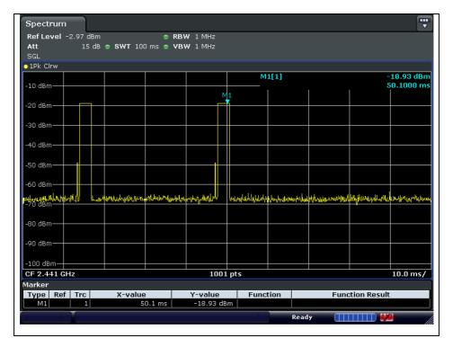
In AFH mode, the minimum hopping frequencies are 20, to get the longest dwell time DH5 packet is observed;
