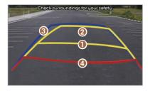
• Driving direction lines (yellow) 102 These lines show the directions of the vehicle according to the steering angle.  Neutral direction lines (blue) These lines indicate your vehicle's expected path with the steering wheel in the neutral position. It can help you determine whether the vehicle is in the
