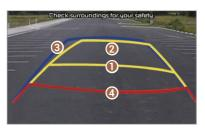
• Driving direction lines (yellow) 10 These lines show the directions of the vehicle according to the steering angle.
