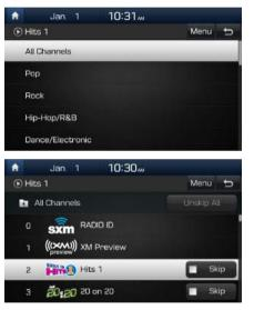
Select the desired category and the channel. Once selected, the previous screen will be restored and the selected channel will begin playing. If you select the Skip button, you can scan channels using the SEEK TRACK key or the TUNE knob by skipping the channels that you chose to skip.
