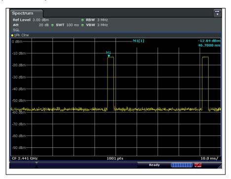
In AFH mode, the minimum hopping frequencies are 20, to get the longest dwell time 3DH5 packet is observed;
