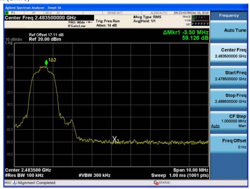
Test Plots with hopping (GFSK) Band Edges (CH.0)
