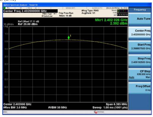
Test Plots (π/4DQPSK) Peak Power (CH.39)
