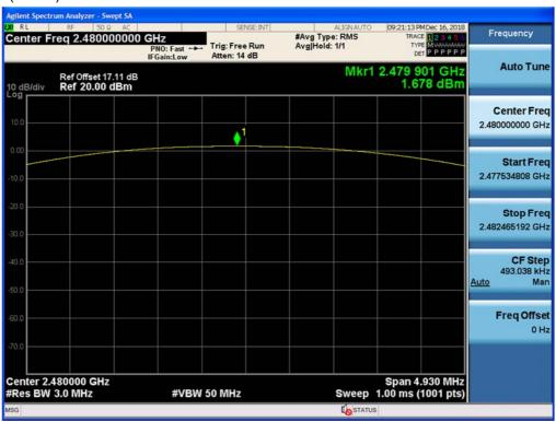
Test Plots (8DPSK) Peak Power (CH.0)
