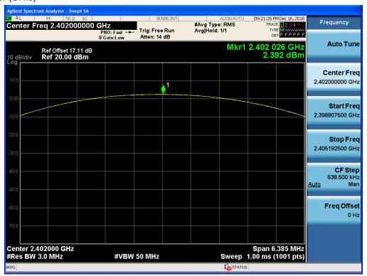
Test Plots (π/4DQPSK) Peak Power (CH.39)
