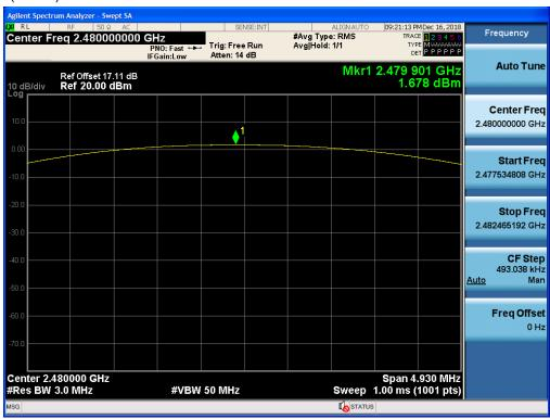
Test Plots (8DPSK) Peak Power (CH.0)
